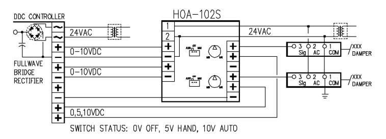
Terminal 2 of the HOA-102S is common to both input and output common (-) terminals. If being used with a controller that utilizes a full wave bridge rectifier in its power supply section (output common is floating or not connected to one side of AC input) an isolation transformer must be used to prevent damage to power supply section.
