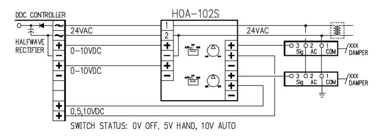
The HOA-102S was designed to provide hand-off-auto with status capability to DDC type controllers in controlling damper position. The HOA-102S can be used for hand-off-auto operations in other applications. Terminal 2 of the HOA-102S is common to both input and output common (-) terminals. The same transformer can be used but polarity must be observed.
